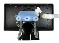
The Quadstick has a joystick, four sip & puff sensors, a lip position sensor, and a push switch connected to a 32-bit ARM processor that converts the sensor inputs into USB and Bluetooth signals for PC's & Game consoles.
